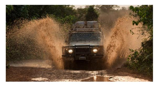
To aid it in conquering Africa's most hostile terrain during its travels, the car was equipped with a number of accessories – which will remain fitted to the vehicle. Reinforced skid plates and nudge bars helped it forge through craggy passes and dense bush. A snorkel intake and mud-terrain tyres gave Holgate confidence through river crossings, dense rain forests and dirt. Off-road shock absorbers allowed for a higher ride-height.
