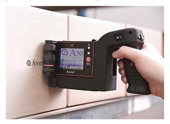
It is hardly surprising that this unique, versatile and lightweight printer is already a hot topic of conversation locally. As the world's lightest and most compact printer, weighing in at a mere 1kg, the U2 Mobile is proving super easy to handle and use on even the most tricky-to-print surfaces.
