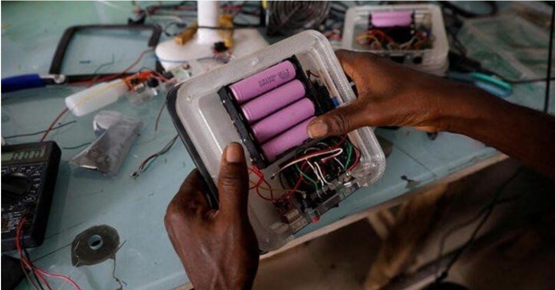
An employee inserts lithium-ion cells from old laptop battery packs into a solar lantern at the Quadloop recycling facility in Lagos, Nigeria. Source: Reuters/Temilade Adelaja
