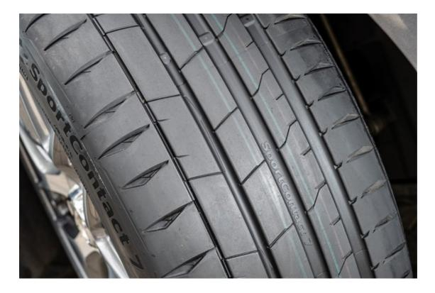
While driving on wet roads, the tyre's footprint ends at the point of the highest water removal in the tread, to offer outstanding grip when braking, accelerating and cornering. When cornering on dry roads, the footprint shifts to the outer shoulder, which is designed to transmit the highest forces for stable handling. New 'locking elements' in the outer shoulder ensure further stability, only enabling limited movement of the tread for high ride stability.
