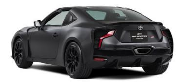
To enhance dynamic performance, the concept has a front-engine, rear-drive layout with the hybrid battery placed centrally for optimal front-rear balance and a low centre of gravity.
