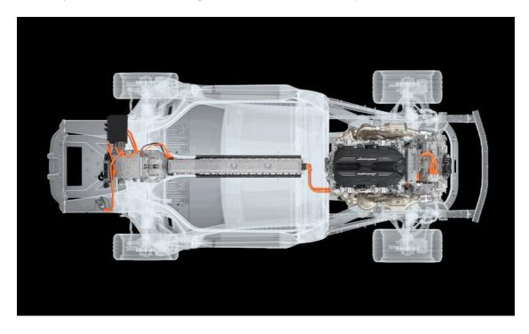
The good news for ICE fans is that the Aventador's replacement will be powered by a V12 engine. However, the naturally aspirated unit will be mated with a trio of electric motors. It is being referred to as the brand's very first high-performance electrified vehicle – (HPEV). The aim of hybridisation is to reduce overall CO2 emissions by 30% when compared to the Aventador Ultimae.
